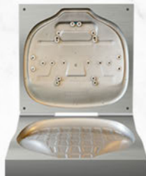
航天钢模具上模内漆 painted in PU steel molding
